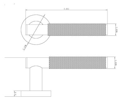
Knurled Lever on rose is a modern design lever on a concealed fix sprung rose. Part of the Eclipse Insignia lever on rose range. Insignia is focuesed on quality and style encompasing modern finishes. Designed for use on residential domestic projects, suitable for architectural specification and DIY merchant markets.
